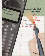
receivers built into whatever computing device you're using—a phone, a hand-held organizer, or a notebook. The data is used to determine the pen's movements based on its x,y coordinates and up/down position and capture your handwriting as "ink." (The technology also works with handwriting recognition software.) InMotion is working with manufacturers to build the technology into all sorts of devices.
