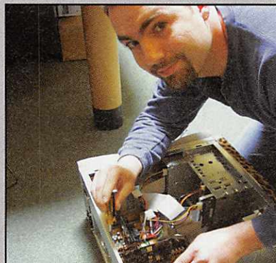
Gallant finds an opening and firmly presses his 3D card into the slot, using a Phillips screwdriver to tighten the screws.
