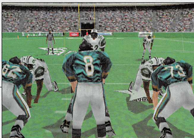
Running on a Voodoo 2 board, the graphics engine renders all 22 characters in 1,200 polygon models.
