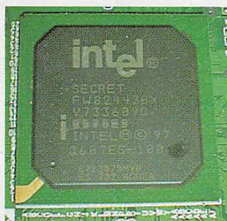
The 440BX core-logic chip, an engineering sample, was marked to ward off curious benchmarkers—like bootBoyz.
