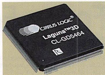
The Laguna3D was designed with Intel's Accelerated Graphics Port in mind.
