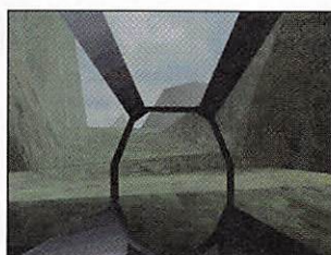
MechWarrior 2 optimized for the Presario 8710's PowerVR 3D graphics accelerator. Note the dithered skyline and the detailed texture mapping used to display terrain elevation.
